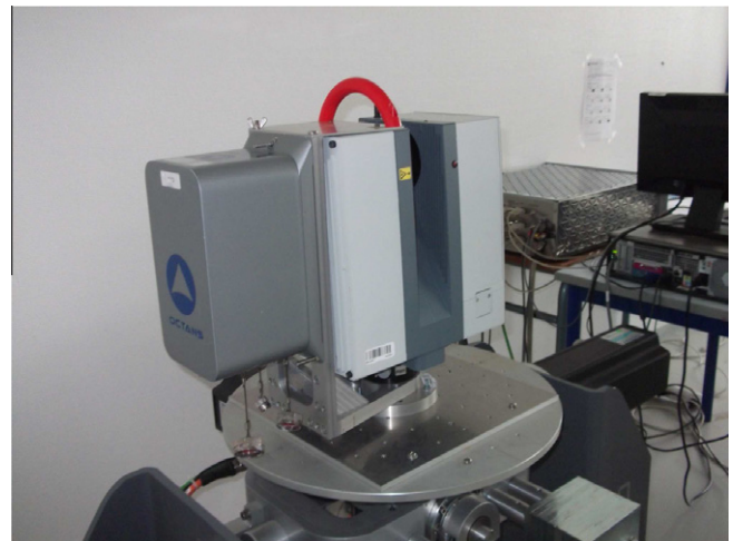
Fig. 3. The system used for latency estimation: a common bracket is used in order to assemble the IMU and the LiDAR. The bracket is mounted on the rotating table. A precision sphere located at 1.5 m away from the LiDAR optical center is used as a target.
